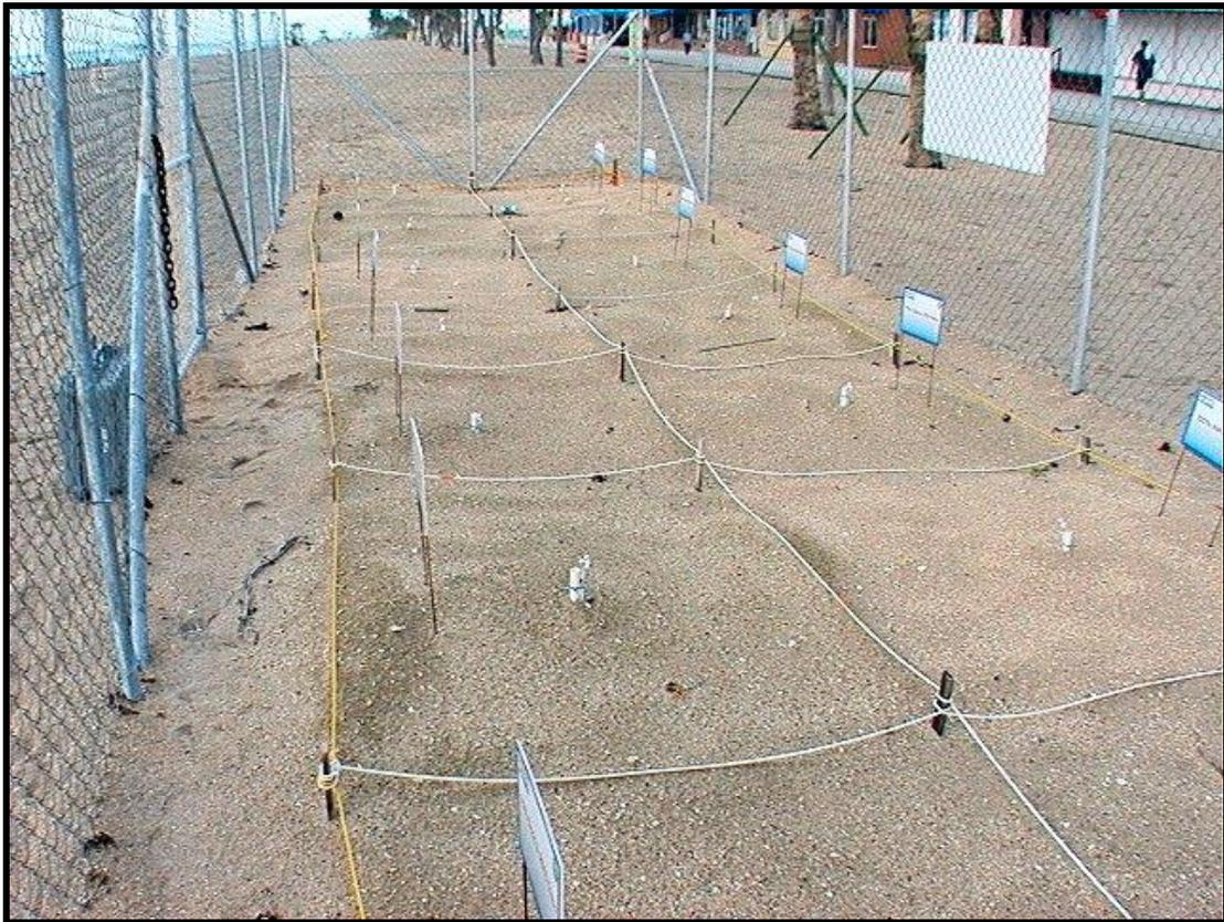
Photo 2. A view of the test plot with the rope demarking varying mixture sections.
